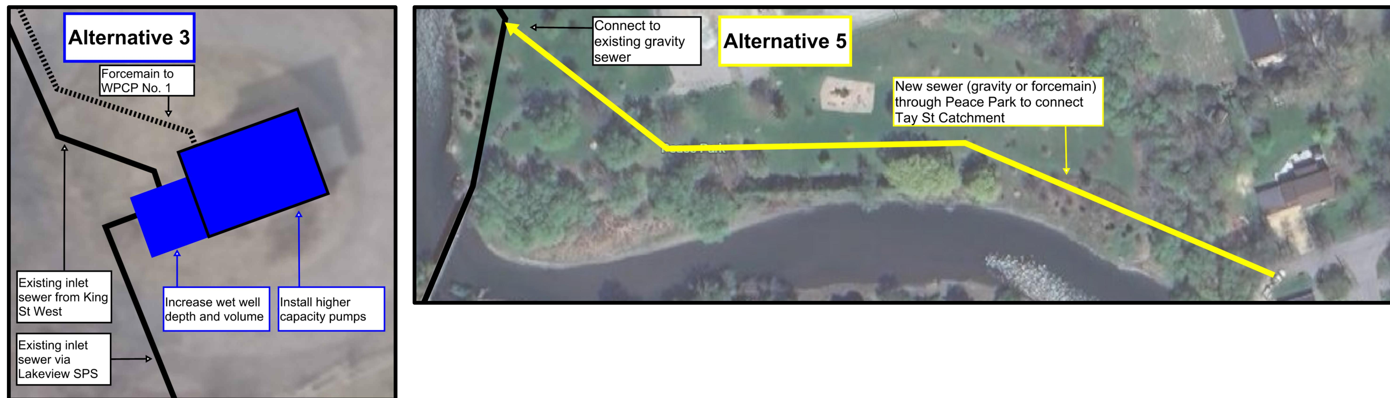
The replacement of forcemain to WPCP No. 1 is also required as part of this solution (alignment to be determined during detailed design in the future).
