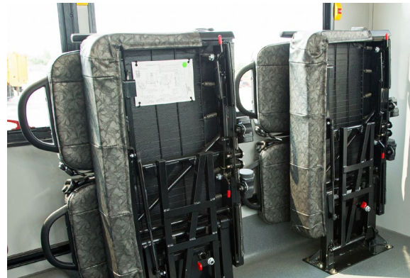
Accessible bus seating, in a folded-up position to provide more space for transit riders.
