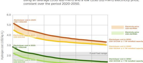
Cost of green hydrogen production as a function of electrolyser deployment, using an average (USD 65/MWh) and a low (USD 20/MWh) electricity price, constant over the period 2020-2050.
