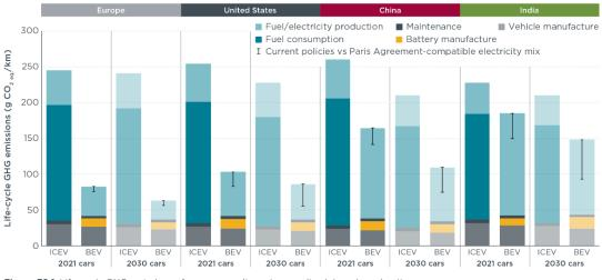
**Figure ES.1**. Life-cycle GHG emissions of average medium-size gasoline internal combustion engine (ICEVs) and battery electric vehicles (BEVs) registered in Europe, the United States, China, and India in 2021 and projected to be registered in 2030. The error bars indicate the difference between the development of the electricity mix according to stated policies (the higher values) and what is required to align with the Paris Agreement.
