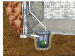
your sump pump. Water from the sump pit is then pumped out and discharged through a pipe in the wall to an outside location far enough from the foundation wall to prevent the discharged water from reentering your foundation drain. The water is then naturally absorbed into the ground. If there is a storm sewer then the sump pit discharge pipe may be directly connected to the storm sewer which discharges the clear water to ditches, creeks and ultimately Lake Ontario.
