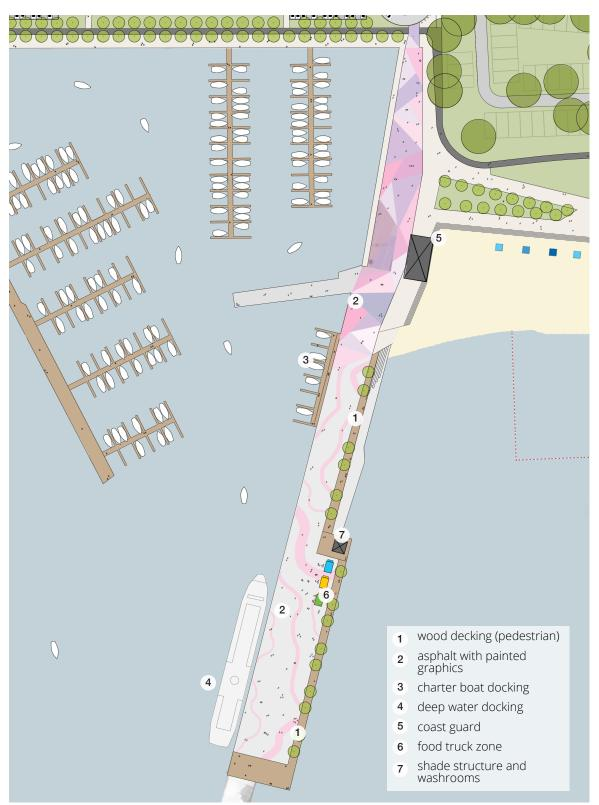
Figure 7.2: East Pier Detailed Design
