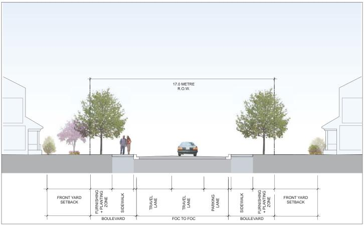
Sample drawing of a typical 2-lane Local Road with a single parking lane and sidewalks adjacent to the curb.
