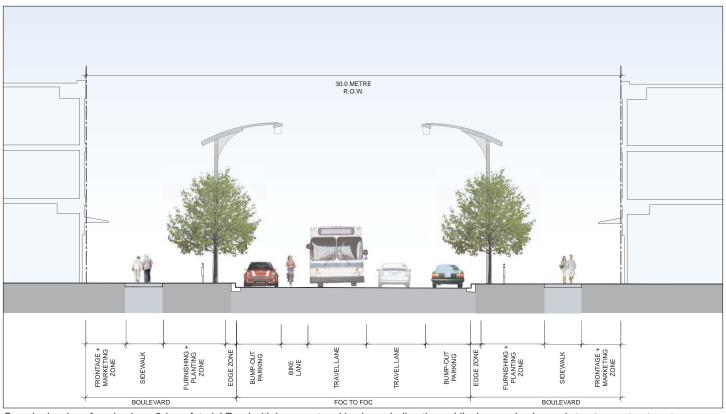
Sample drawing of a mixed use 2-lane Arterial Road with bump-out parking in each direction, a bike lane and enhanced streetscape treatments.
