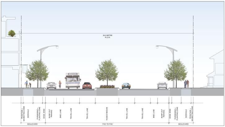
Sample drawing of a 4-lane mixed use Arterial Road with a central median, bump-out parking and bike lanes in each direction.
