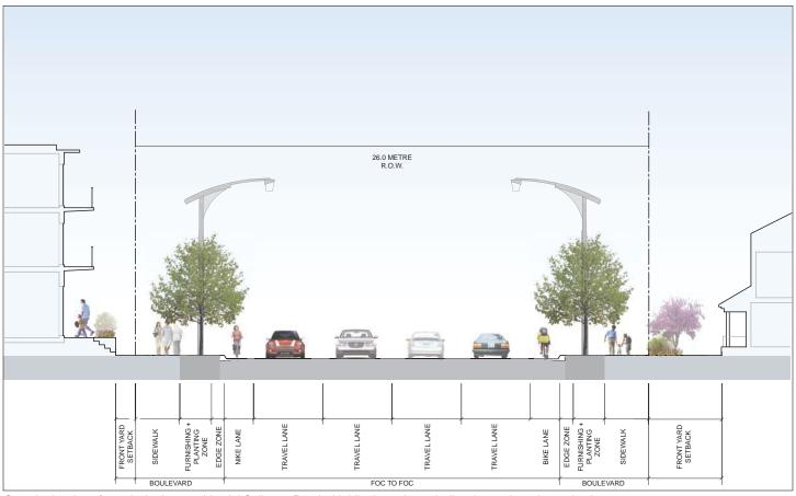
Sample drawing of a typical 4-lane residential Collector Road with bike lanes in each direction and varying setbacks.
