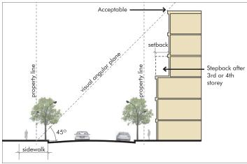
The Visual Angular Plane Analysis is used as one means to determine building mass and adjacent site impacts as the building height increases.
