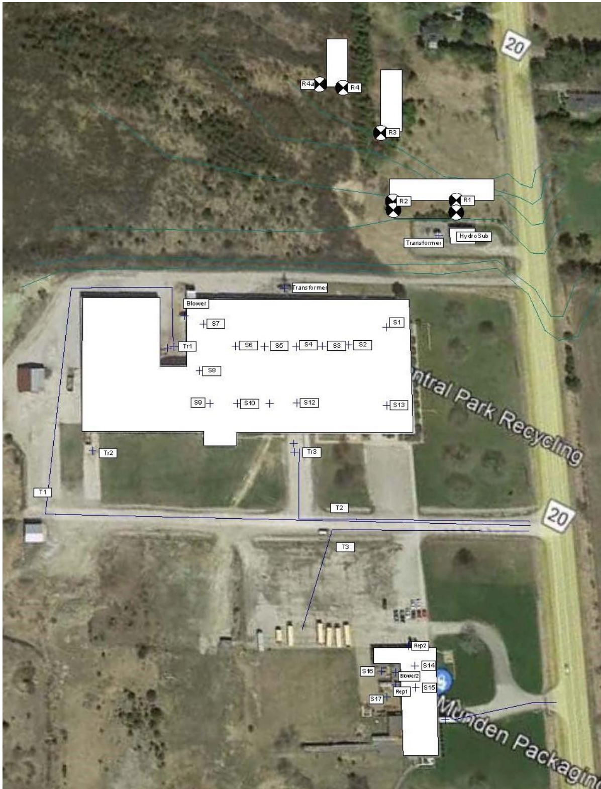
FIGURE 5 Cobourg Trails (Phase 2) LOCATION OF STATIONARY NOISE SOURCES (CadnaA)
