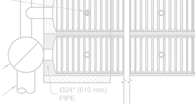
The ChamberMaxx system combines middle chambers, which are open on both ends, with start and end chambers, which include an integral end wall. Water is stored in both the chamber and in the void space in the surrounding stone backfill providing 75.1 cubic feet of storage per chamber. The ChamberMaxx system can be configured with up to 24-inch diameter (0.61 m) inlet/outlet manifold.
