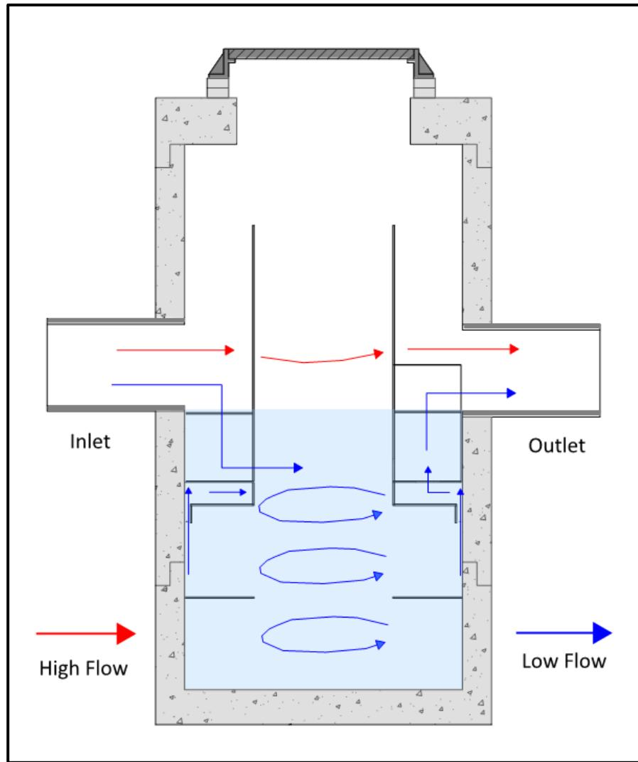
**Figure 2. Hydroworks HydroStorm Operation – Profile View**
