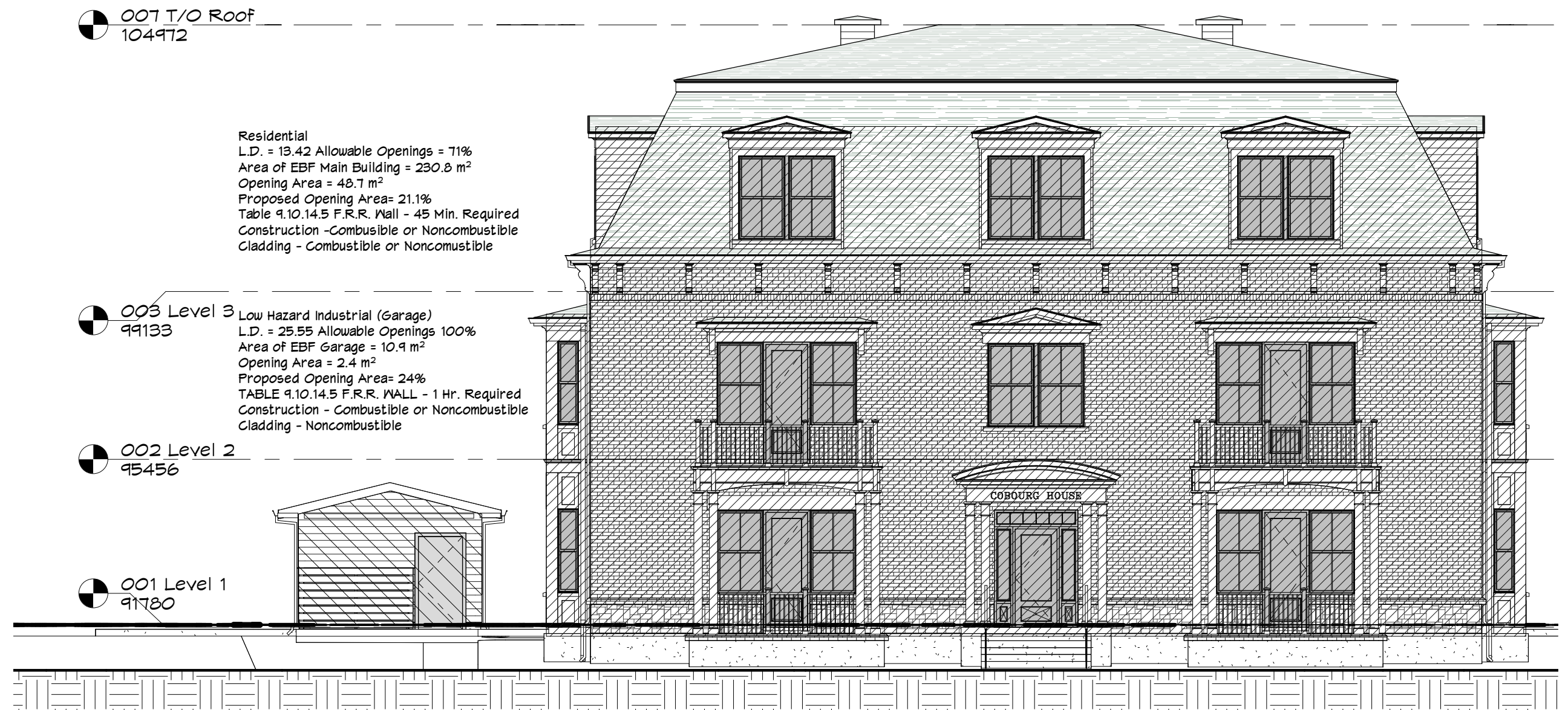
1 Limiting Distance - North Elevation A1.1 1: 100
