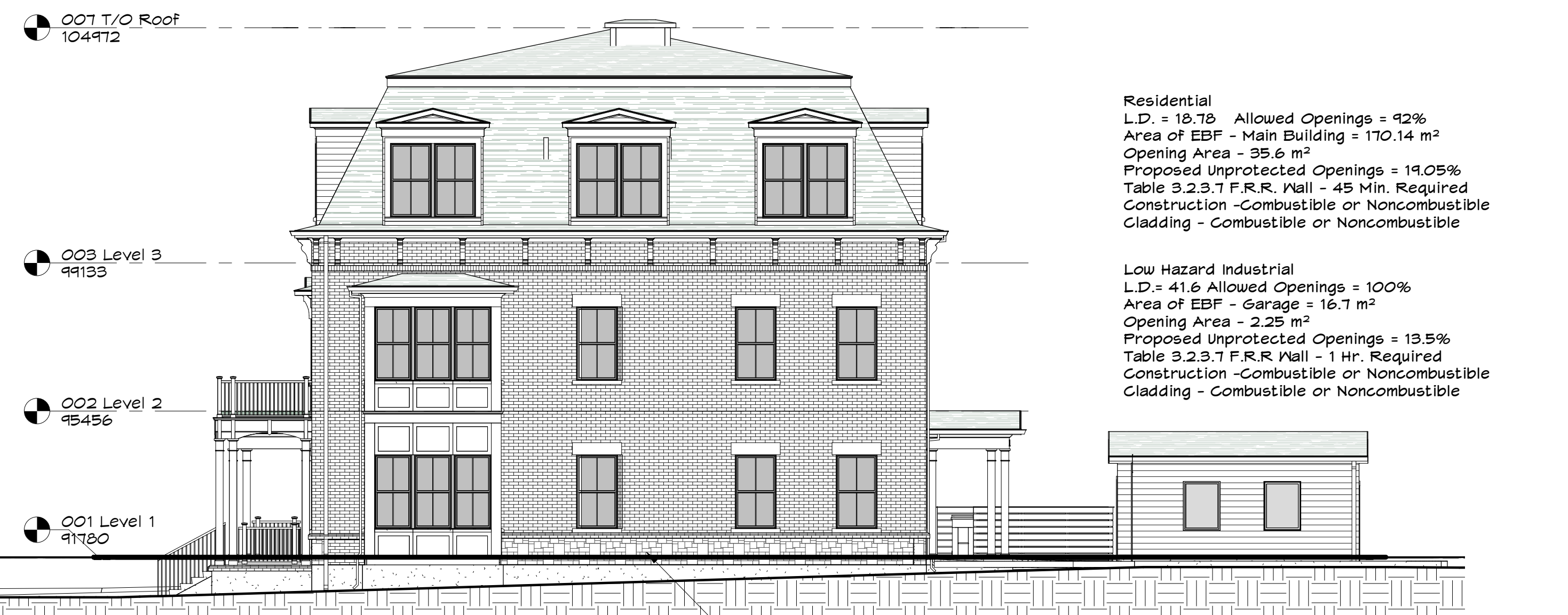
4 Limiting Distance - West Elevation A1.1 1: 100
