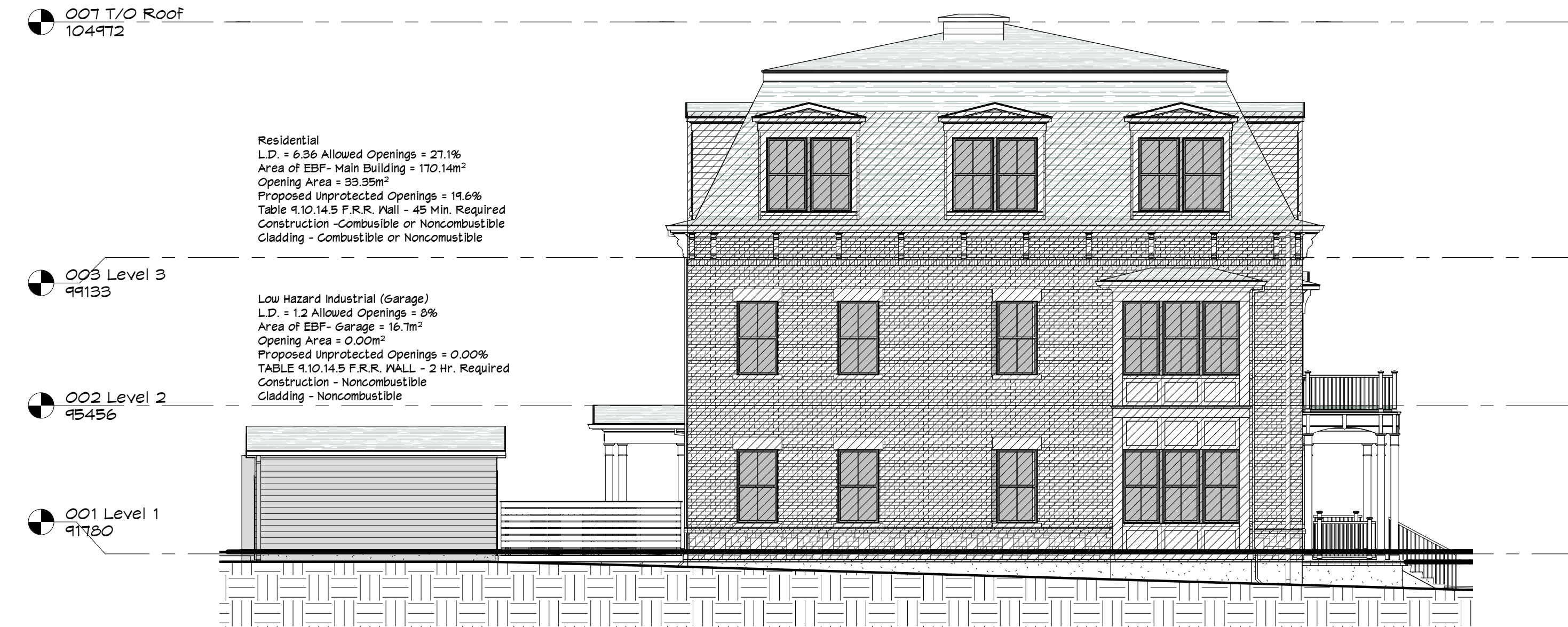
2 Limiting Distance - East Elevation A1.1 1: 100
