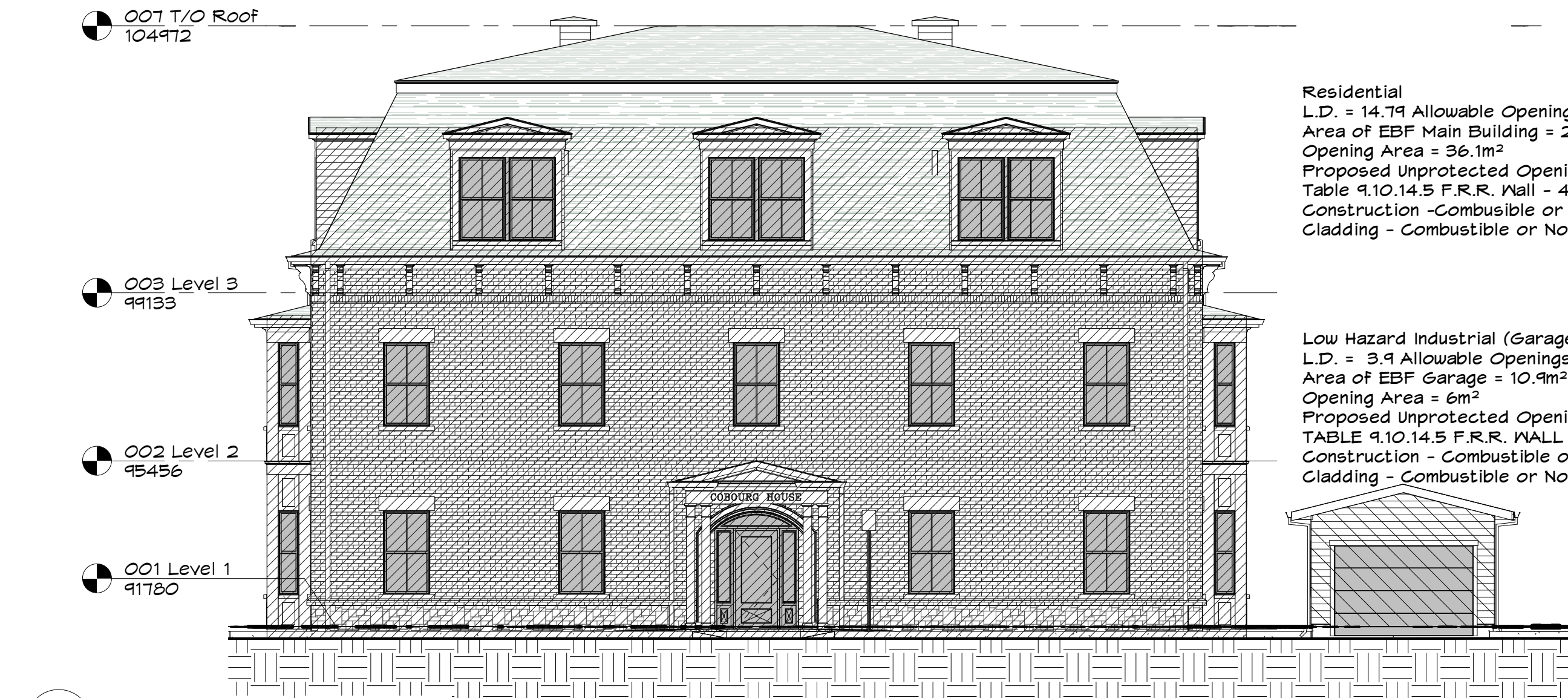
3 Limiting Distance - South Elevation A1.1 1: 100
