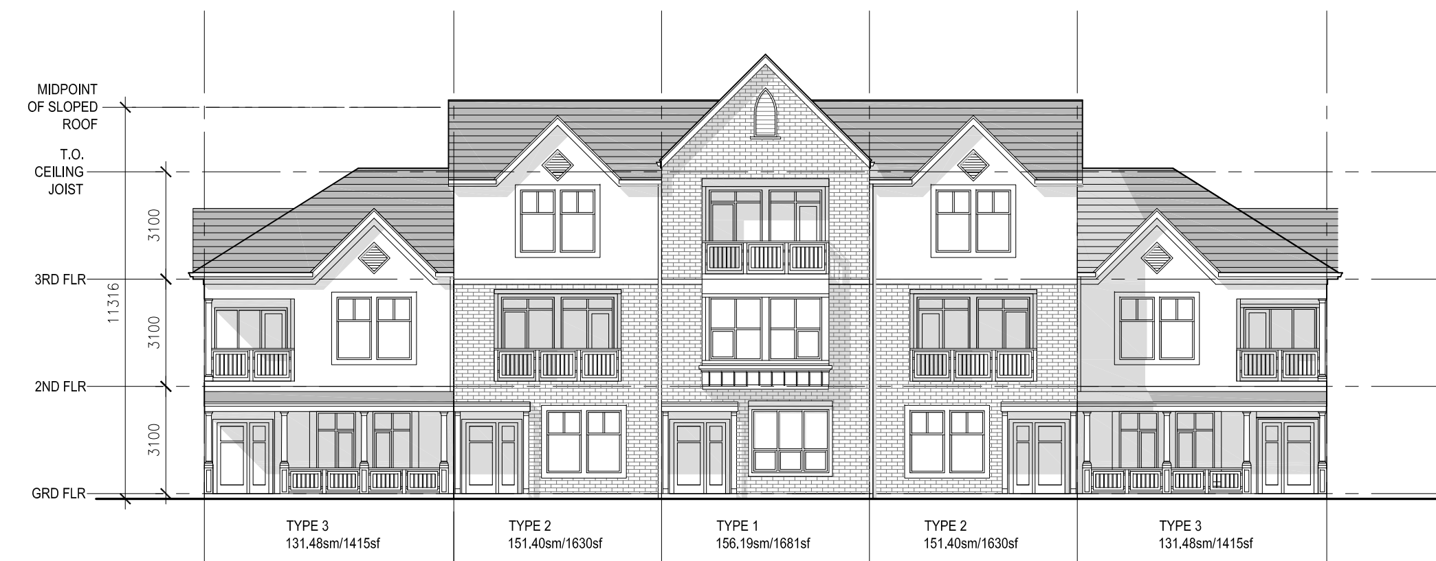
2A SOUTH ELEVATION - FRONT A1 BLOCK B
