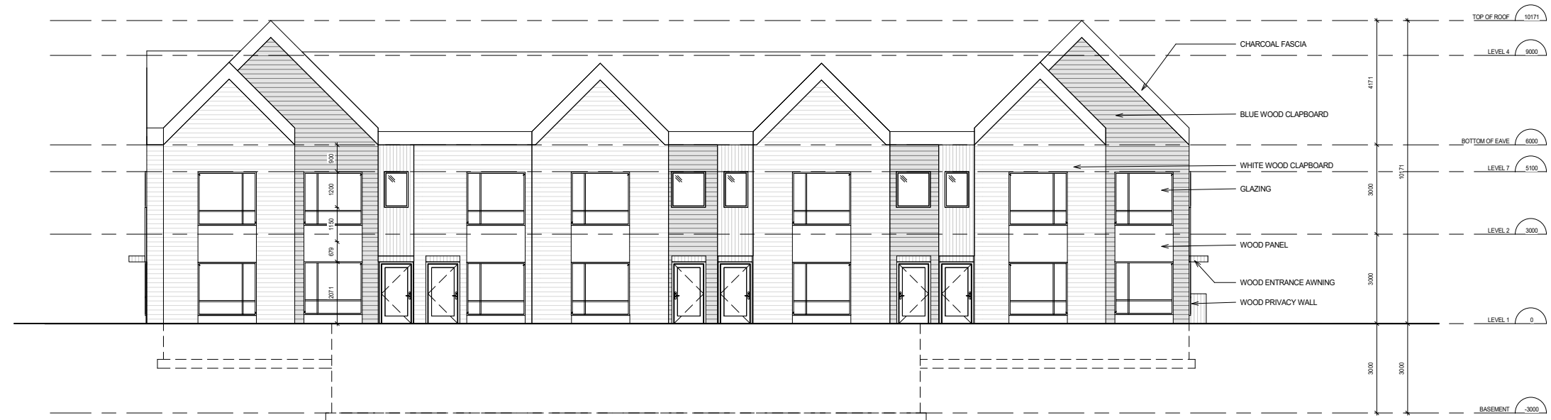
1 A009 SOUTH ELEVATION TYPICAL BUILDING BURNET DR. 1:75
