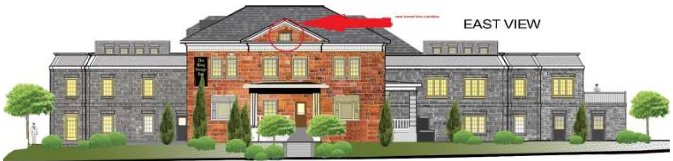
Above: Plan for new dormer windows and skylights (east view)
