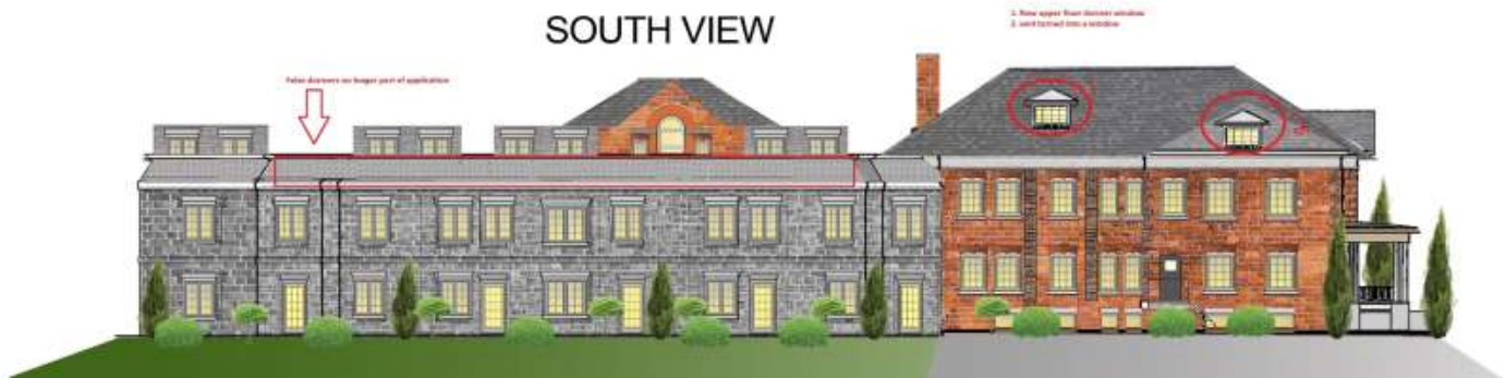
Above: Plan for new dormer windows and skylights (south view)
