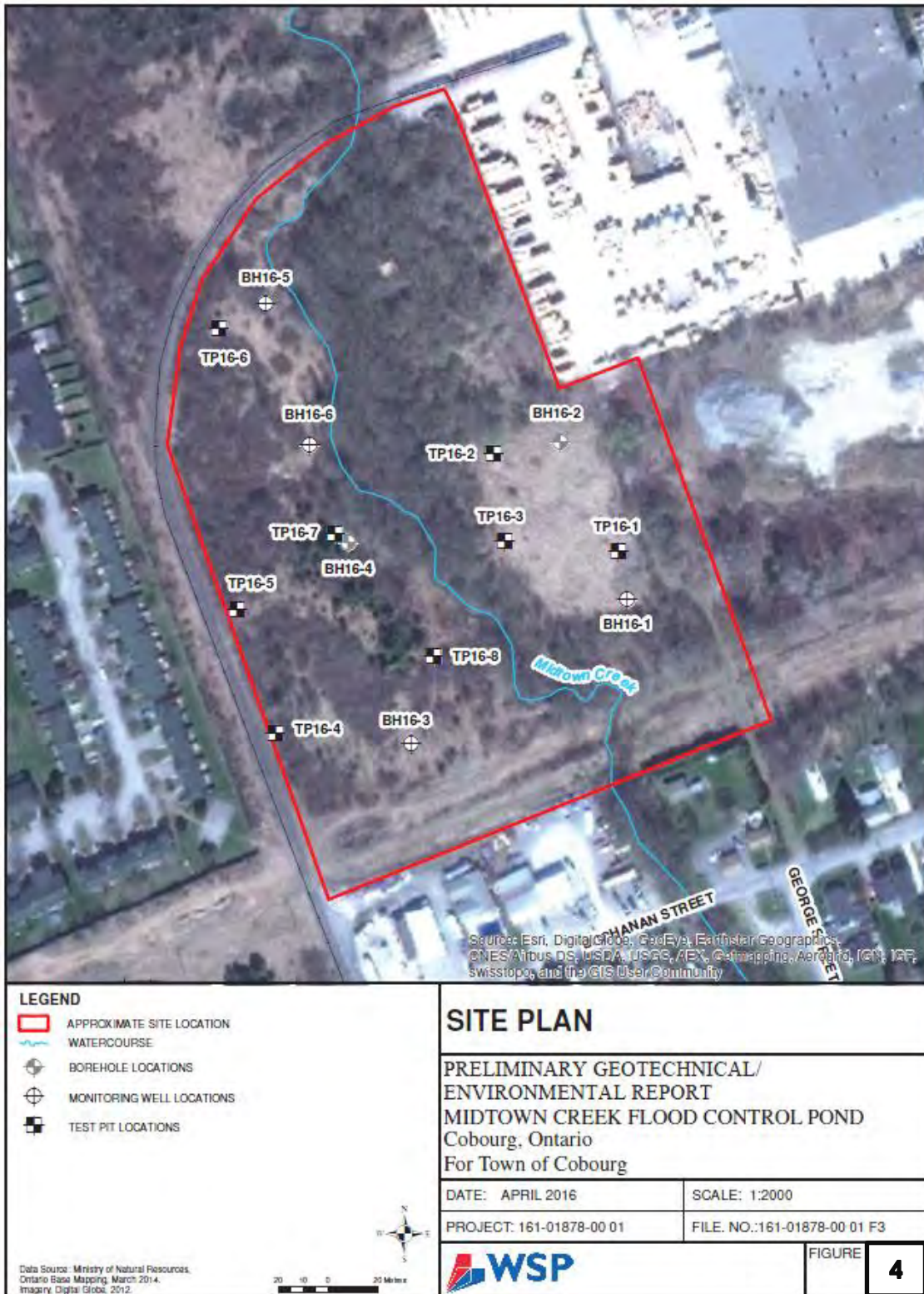
Figure 4 – Borehole and Test Pit Locations (WSP 2016)
